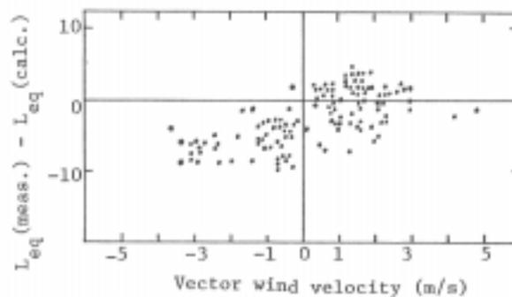
Fig. 11 Effect of wind on the propagation of road traffic noise
