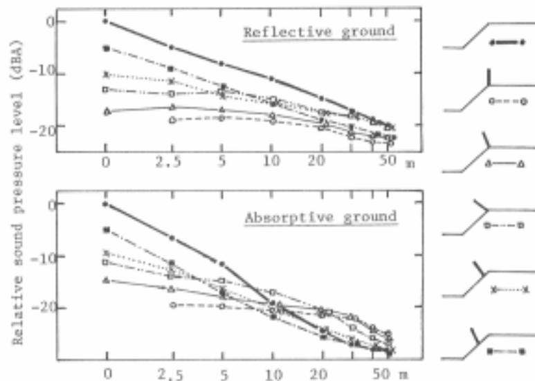
Fig.7 Effect of the barrier configurations on the propagation of noise from depressed road
