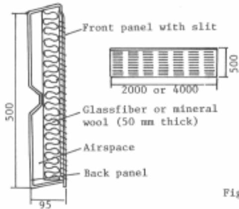
Fig.1 Section and front view of a standard panel
