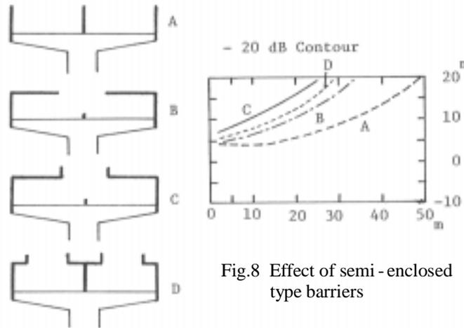
Fig.8 Effect of semi - enclosed type barriers
