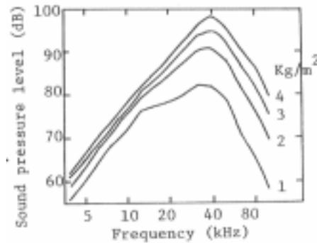
Fig.4 Spectrum of jet noise at 30 cm from the line source.
