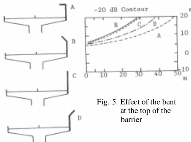
Fig. 5 Effect of the bent at the top of the barrier
