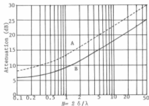
Fig.3 Sound attenuation by acoustic barrier
