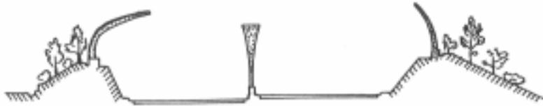
Fig. 10 Sectional view of specially shaped barrier
