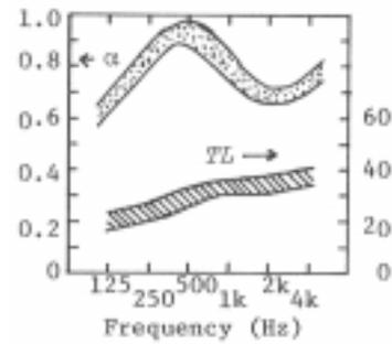
Fig.2 Acoustic characteristics of standard panel
