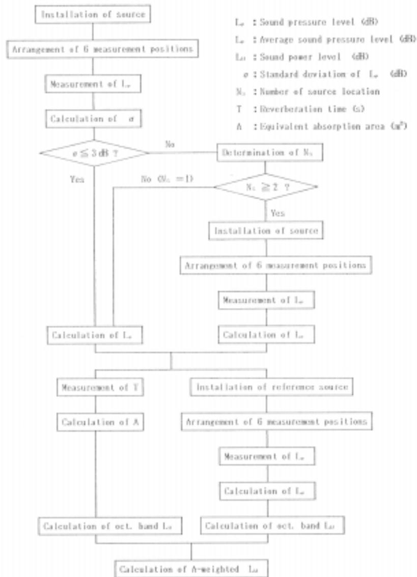
Fig.3 Measurement procedure for the survey diffuse field method (JIS Z 8733 Method C).
