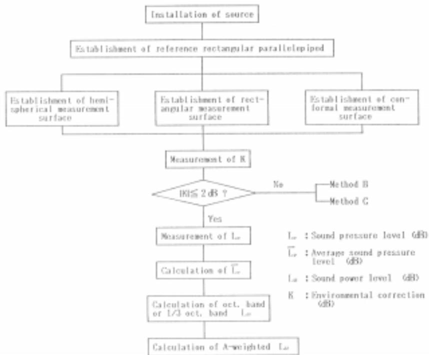
**Fig.1** Measurement procedure for the engineering hemi-free field method (JIS Z 8733 Method A).
