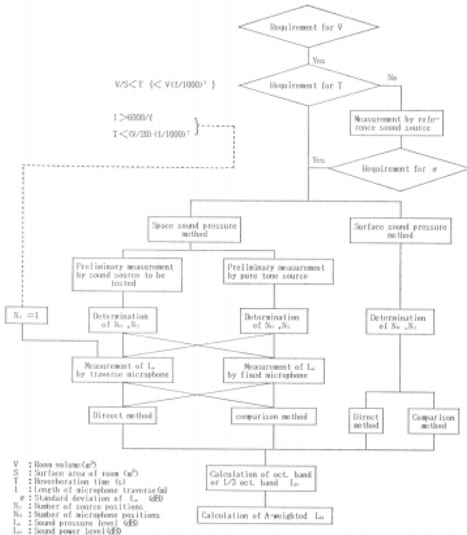
**Fig.4** Measurement procedure for the precision diffuse field method (JIS Z 8734).
