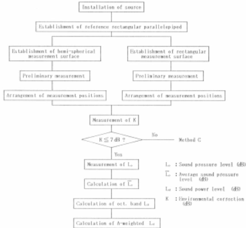
Fig.2 Measurement procedure for the survey hemi-free field method (JIS Z 8733 Method B).
