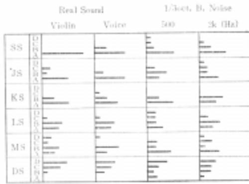
Fig. 3-1 Results of the study on the elevation of the perceived orbit at the direction of 0 deg. for various combinations of "head" and "listener". SS: recorded by the listener's head, JS-MS: the head of different person, DS: the unmodified dummy head.
