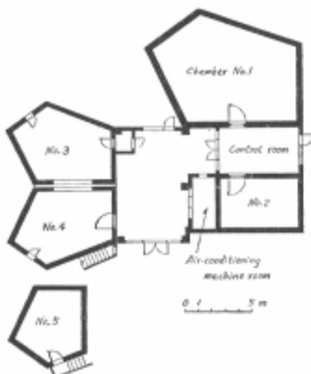
FIG. 1. Plan of the five reverberation chambers used for the measurements of the sound absorption coefficient and the transmission loss.
