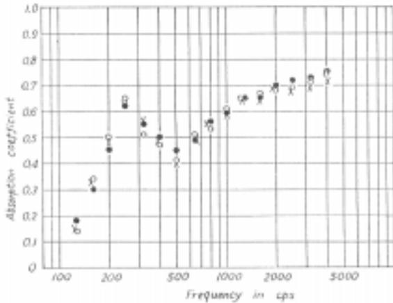
FIG.6. Effect of the position of test specimens on the absorption coefficient. floor center, floor edge, x floor and two walls.
