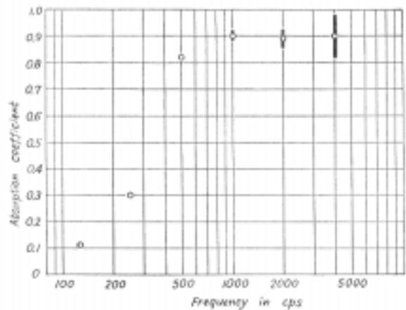
FIG.5. Effect of the microphone position on the absorption coefficient of test specimens. Lines show the deviation of absorption coefficient when one microphone moves to seven positions and twenty decay curves are measured at each position.
