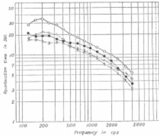
FIG.3. Reverberation times of five reverberation chambers without test specimens. — - chamber No.1, - - - - - No.2, . . . . No.3 and No.4, - · · · - No.5.
