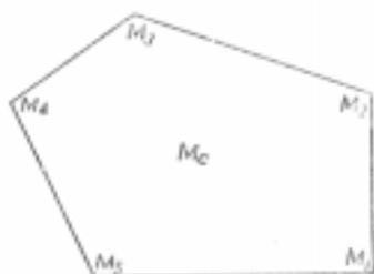
Fig. 7. Positions of microphone for reverberation measurements.
