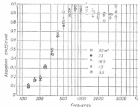
Fig. 12. Effect of sample area on absorption coefficient of mineral wool.
