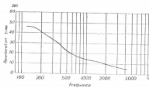
Fig. 6. Reverberation times for empty chamber.
