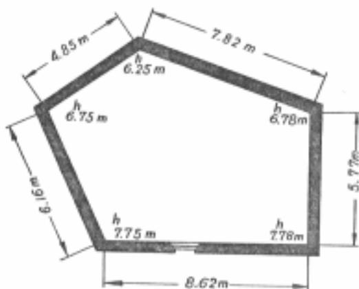
Fig. 1. Plan of the reverberation chamber.  $h$  shows the height of each corner.
