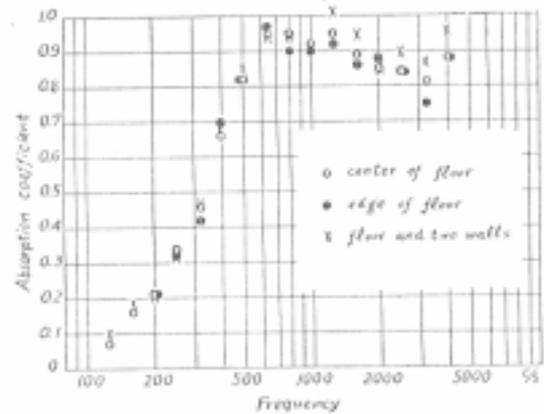
Fig. 14. Effect of sample position on absorption coefficient of mineral wool. Sample area 10m<sup>2</sup>.
