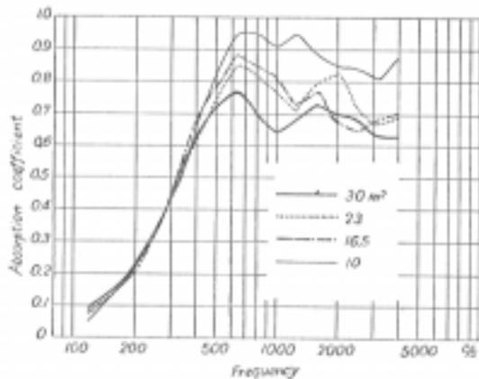
Fig. 16. Effect of sample area on absorption coefficient of mineral wool (sample placed on the floor only)
