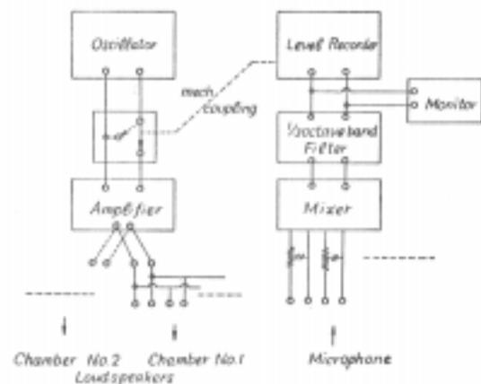
Fig. 3. Block diagram of the apparatus for the measurements of reverberation time.
