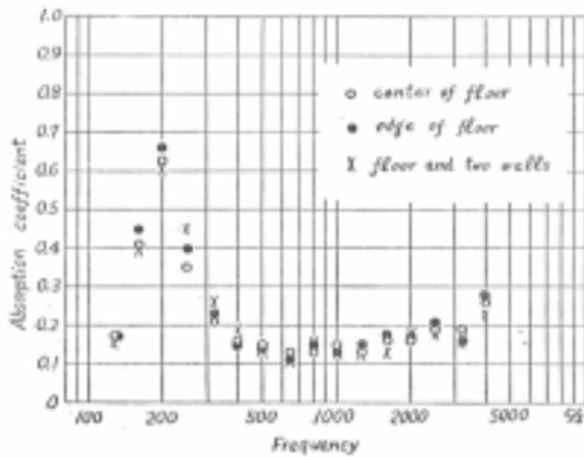
Fig. 13. Effect of sample position on absorption coefficient of fibrous acoustic tiles. Sample area 10m<sup>2</sup>.
